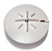
Addressable heat (58 °C fixed temperature and thermal rate of rise) detector with builtin isolator, with algorithm verification. Led status indicator and output for remote pilot or buzzer, anti-theft system. White color. Requires base Z-200 or Z-200-H. CPR certificate EN54-5 and EN54-17. Dimensions: 100 x 40 mm.
