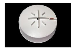
**Addressable high temperature detector (fixed at 78°C),** with algorithm verification. Led status indicator and output for remote pilot or buzzer, anti-theft system. White color. Allows installation without polarity. Requires connection base Z-200 or Z-200-H. CPR certificate EN54-5. Dimensions: 100 x 40 mm.
