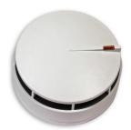
**Addressable optical smoke detector,** with dirt compensation and algorithm verification. Led status indicator anti-theft system and output for remote pilot indicator PAD-10 or buzzer BUD-200. White color. Non polarity installation. Requires connection base Z-200 or Z-200-H. CPR certificate EN54-7. Dimensions: 100 x 40 mm.
