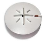
Addressable high temperature detector (fixed at 78°C) with built-in isolator, with algorithm verification. Led status indicator and output for remote pilot or buzzer, anti-theft system. White color. Requires connection base Z-200 or Z-200-H. CPR certificate EN54-5 and EN54-17. Dimensions: 100 x 40 mm
