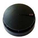
**Addressable optical smoke detector,** with dirt compensation and algorithm verification. Led status indicator anti-theft system and output for remote pilot indicator PAD-10 or buzzer BUD-200. Black color. Non polarity installation. Requires connection base Z-200 or Z-200-H. CPR certificate EN54-7. Dimensions: 100 x 40 mm.
