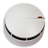
Addressable optical smoke detector with built-in isolator, with dirt compensation and algorithm verification. Led status indicator anti-theft system and output for remote pilot indicator PAD-10 or buzzer BUD-200. White color. Requires connection base Z-200 or Z-200-H.
