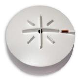
Addressable heat (58°C fixed temperature and thermal rate of rise) detector, with algorithm verification. Led status indicator and output for remote pilot or buzzer, anti-theft system. White color. Allows installation without polarity. Requires base Z-200 or Z-200-H. CPR certificate EN54-5. Dimensions: 100 x 40 mm.
